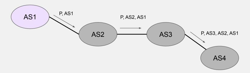
An AS could also add its ASN multiple times to the AS Path, doing what we call AS Path Prepending, to make the path less desirable: e.g., for more expensive routes, backup link.
